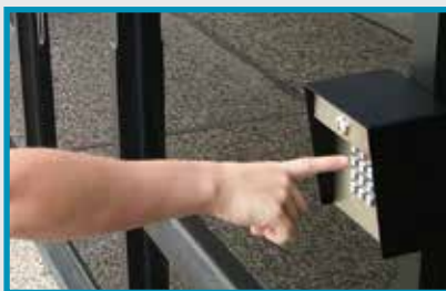
Digital Keypad Code Entry Enter 4 or 5-digit unique PIN to gain entry, up to 1000 4-digit entry codes
