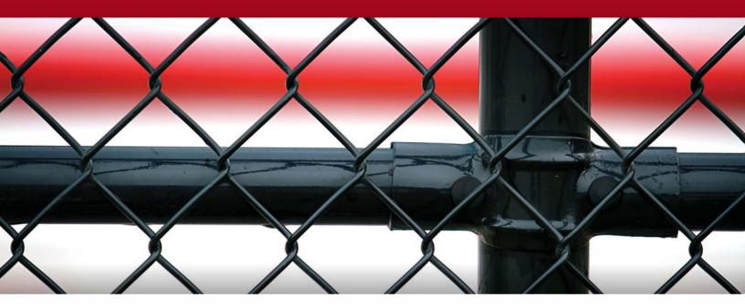
Wheatland Tube's WT-ColorCoat for fence framework offers four layers of protection. The galvanized coating, intermediate conversion coating, clear polymer coating and polyester coating together make WT-ColorCoat attractive, durable and dependable.
